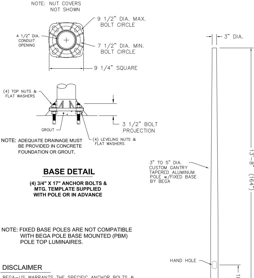
BEGA-US WARRANTS THE SPECIFIC ANCHOR BOLTS & POLE COMBINATION ACCORDING TO THE PRODUCT NUMBER(S) AND DESCRIPTIONS(S). STRUCTURAL CHANGES TO THE POLE REQUESTED BY THE CUSTOMER INCLUDING CHANGES TO POLE LENGTH, MAY AFFECT THE COMPATIBILITY OF THE ANCHOR BOLTS AND CORRESPONDING POLES.
