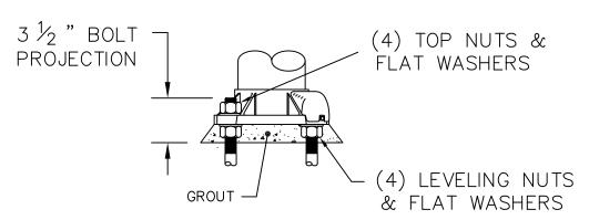
NOTE: ADEQUATE DRAINAGE MUST BE PROVIDED IN CONCRETE FOUNDATION OR GROUT.
