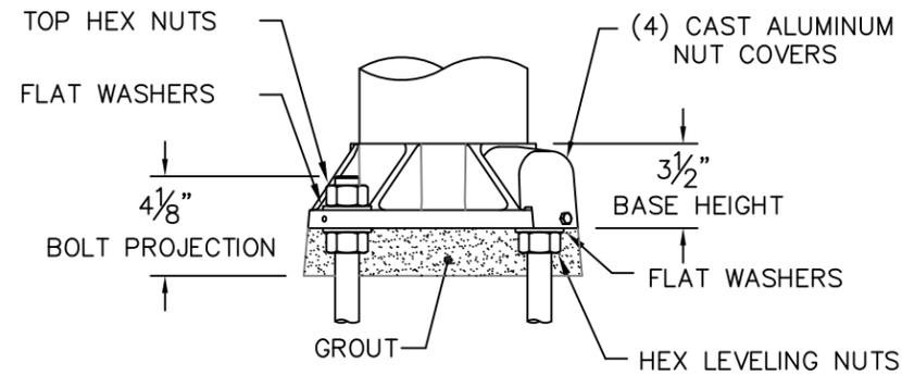
NOTE: ADEQUATE DRAINAGE MUST BE PROVIDED IN CONCRETE FOUNDATION OR GROUT.
