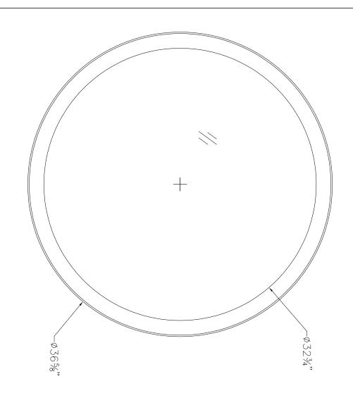
NOTES: 1. LUMINAIRE # 24 231 — SEE SPECIFICATIONS 2. FIXTURE MUST BE WIRED DIRECTLY TO ½" NPT THREADED WIREWAY BASE
