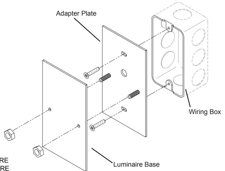
**IMPORTANT:** note position of orientation arrow on luminaire base and install accordingly.
