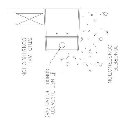
ISOMETRIC VIEW INSTALLATION HOUSING (NOT TO SCALE)
