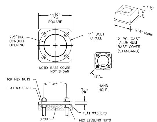
NOTE: ADEQUATE DRAINAGE MUST BE PROVIDED IN CONCRETE FOUNDATION OR GROUT.
