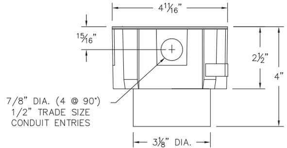
**SMALL OPENING WIRING BOX DETAIL**
