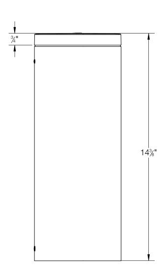
71126 SYSTEM BOLLARD HEAD SHOWN ON SYSTEM BOLLARD TUBE 99614 (NOT TO SCALE, TUBE SOLD SEPERATELY)
