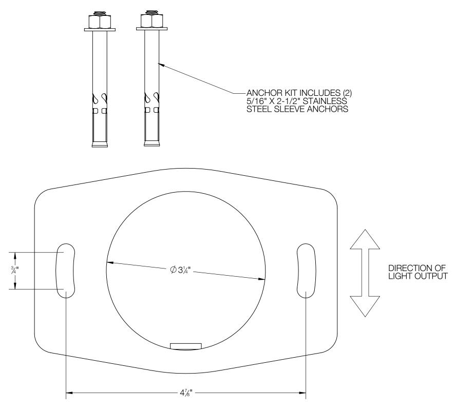
NOTE: ANCHOR KIT DOES NOT INCLUDE TEMPLATE, USE BOLLARD BASE AS TEMPLATE (SHOWN)
