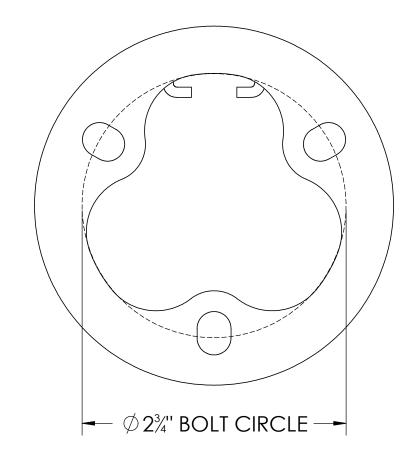
NOTE: ANCHOR KIT DOES NOT INCLUDE TEMPLATE, USE BOLLARD BASE AS TEMPLATE (SHOWN)
