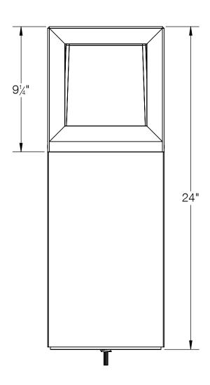
84681 SYSTEM BOLLARD HEAD SHOWN ON SYSTEM BOLLARD TUBE 84001 (NOT TO SCALE, TUBE SOLD SEPERATELY)
