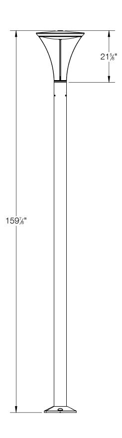
84735 SYSTEM BUILDING ELEMENT HEAD SHOWN ON SYSTEM BUILDING ELEMENT POLE 84709 (NOT TO SCALE, POLE SOLD SEPERATELY)
