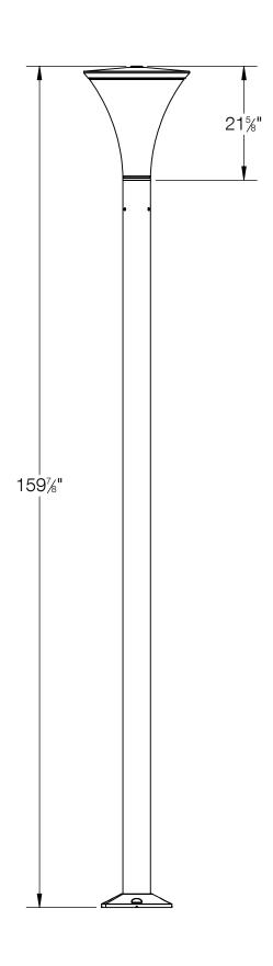
84737 SYSTEM BUILDING ELEMENT HEAD SHOWN ON SYSTEM BUILDING ELEMENT POLE 84709 (NOT TO SCALE, POLE SOLD SEPERATELY)
