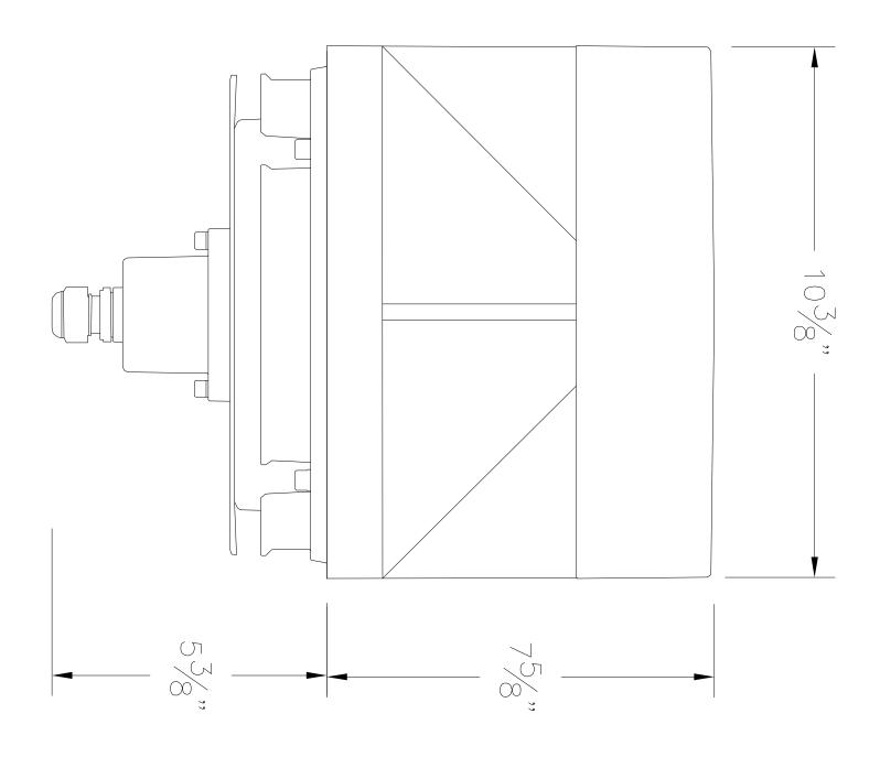
99 777 Shown on Bollard Tube 99 619 (SCALE 1:2)
