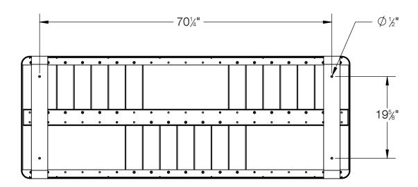
NOTE: INCLUDES SLEEVE ANCHOR KIT FOR SECURING TO FINISHED CONCRETE
