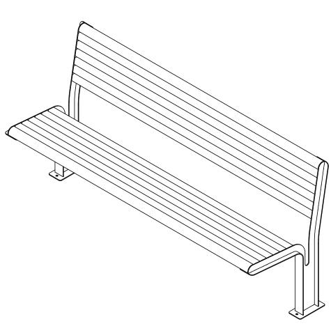
NOTE: INCLUDES SLEEVE ANCHOR KIT FOR SECURING TO FINISHED CONCRETE
