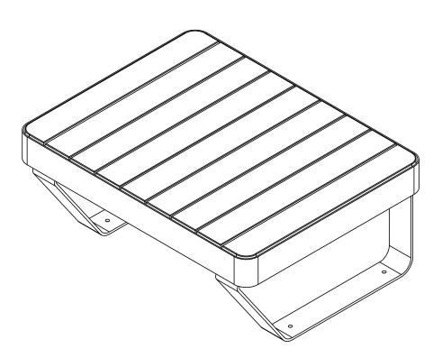
NOTE: INCLUDES SLEEVE ANCHOR KIT FOR SECURING TO FINISHED CONCRETE
